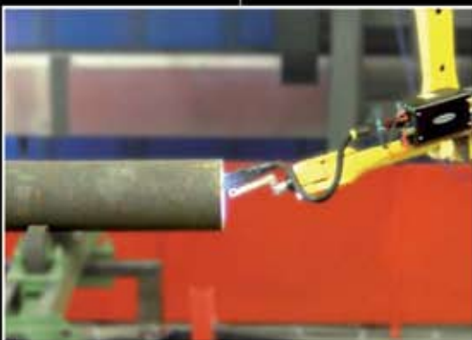
CLADDING OF PIPE
