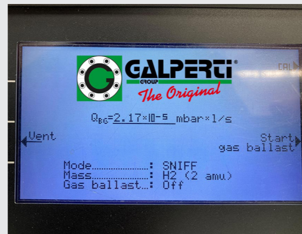
Testing facility equipped to perform seat gas test and fugitive emission test with blend 95% Nitrogen with 5% Hydrogen.
